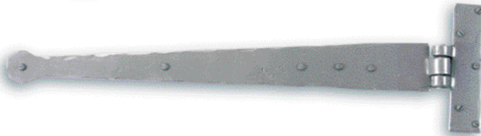
03-060-02 Weighty Scotch Pattern Tee Hinge 470mm x 130mm overall. Hinge Front 420mm. Butt 130mm x 35mm.
